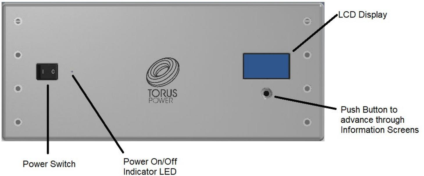
The front panel consists of a 4 line LCD display and a pushbutton switch. Each time you push the button the display will show a different feature of the AVR ELITE.
