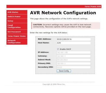
Each AVR unit has a unique MAC Address which is factory assigned.
