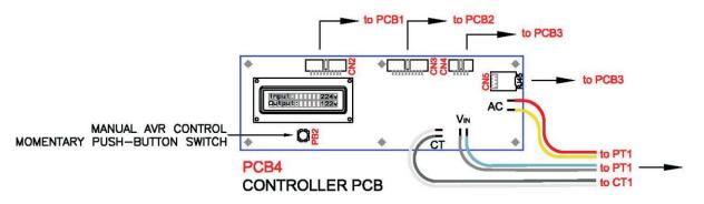
Automatic Voltage Regulation - Controller PCB with digital display (display is drawn mirrored), fastened to the inside of the enclosure door.
