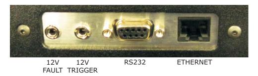
Figure 1: AVR Rear Panel connections.
