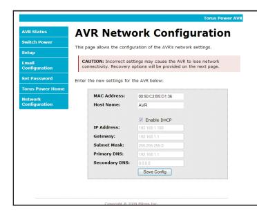
Each AVR unit has a unique MAC Address which is factory assigned.
